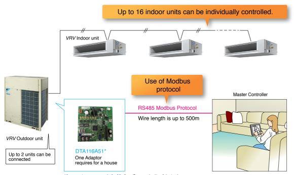
\*A separate power supply for Modbus Communication Adaptor is necessary. It may not be installed inside some outdoor unit models.
