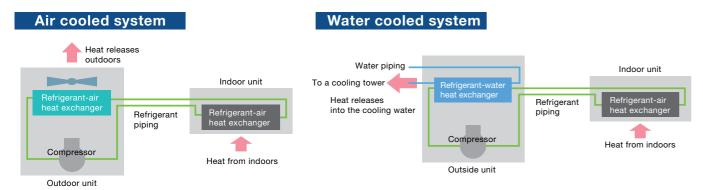
As a water cooled system does not require to exchange heat with outdoor air,
