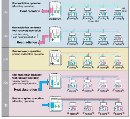
Note: Operation modes (A) and (E) are applicable when the outdoor temperature is 35°C and 7°C respectively; The other modes are applicable under typical outdoor conditions.
