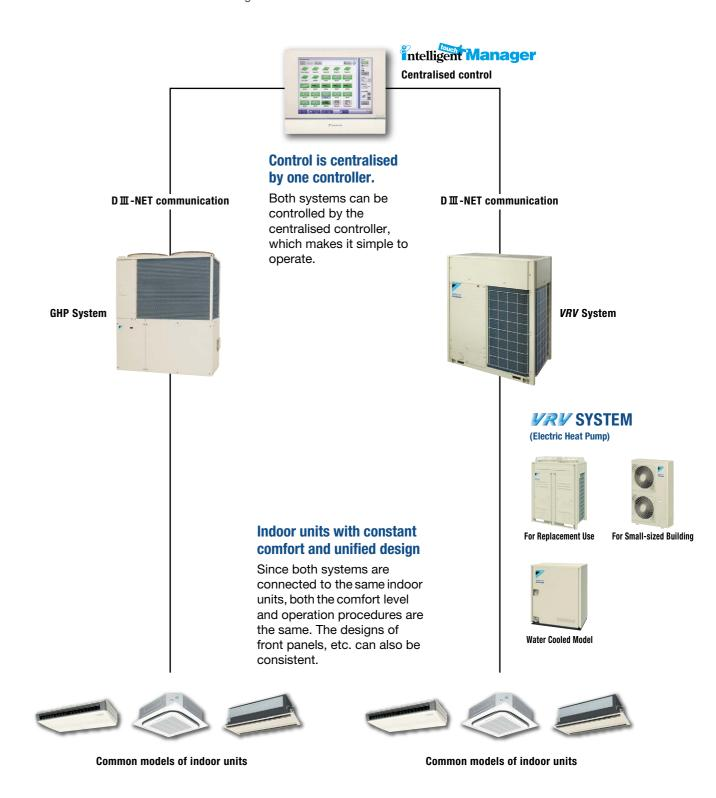
Common indoor models for both GHP and EHP systems ensure a consistent look for exposed units whilst maintaining similar comfort levels and keeping operational control.
