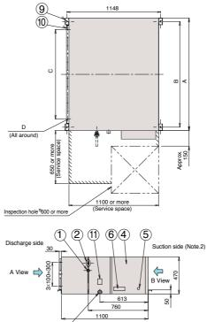
\*These diagrams are based on FXMQ200 and FXMQ250MFV1.
