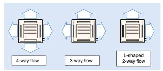
For 3-way or 2-way flow installation, the sealing material for air discharge outlet
