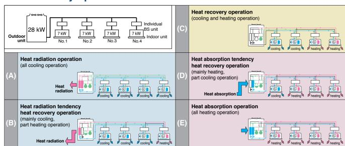
Note: Operation modes (A) and (E) are applicable when the outdoor temperature is 35°C and 7°C respectively; The other modes are applicable under typical outdoor conditions
