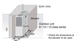
The compact outdoor unit can be installed on the service balcony of each floor.
