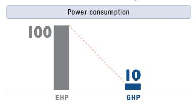
In GHP system, only the condenser fans and the indoor units consume electricity. In comparison to EHP, the electrical power required to operate GHP is significantly less, thereby enabling the electrical substation and switch gear equipment to be downsized compared to EHP.
