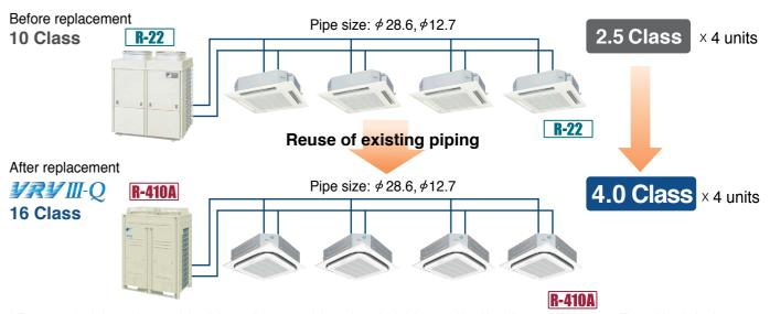
\* For reuse of existing refrigerant piping, it is possible to use piping or branched piping capable of handling 3.3 MPa or more. Thermal insulation is necessary for liquid piping and gas piping.
