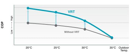
Required capacity changes as air conditioning load changes according to outdoor temperature.
