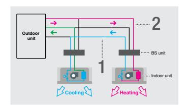
The (cold) waste heat from heating is used for the cooling operation.
