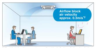
Airflow block function prevents uncomfortable drafts by reducing air velocity to approx.  $0.3 \, \text{m/s.}^{*2}$
