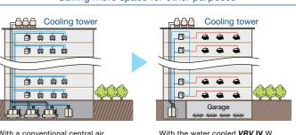
With a conventional central air conditioning system, the outside units take up a disproportionately large amount of space for installation.
